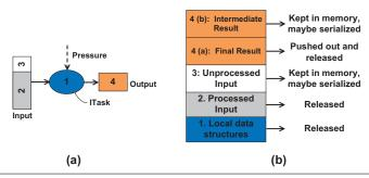
**Figure 1.** A graphical illustration of (a) an ITask execution at an interrupt with numbers showing different components of its memory consumption; and (b) how these components are handled.
