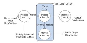
**Figure 5.** The data flow of an ITask execution.
