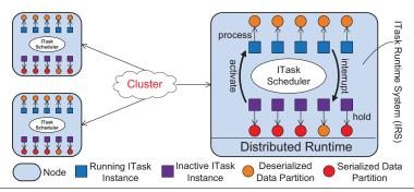
**Figure 2.** The architecture of the ITask Runtime System.
