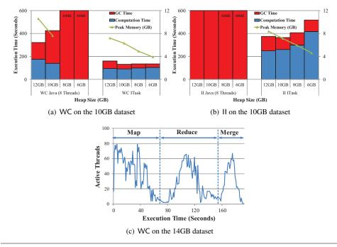
**Figure 11.** (a) and (b) show how performance changes as we vary the heap size; (c) shows how the number of active ITask instances changes as the execution progresses.
