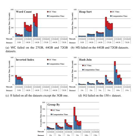
**Figure 9.** Performance changes as we vary thread number in the original programs; the task granularity is 32KB.
