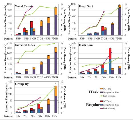
**Figure 10.** Comparisons between the ITask versions (the second/right bar in each pair) and their Java counterparts with the best configurations (the first/left bar). Each error bar represents the standard deviation of the times collected from 5 runs.
